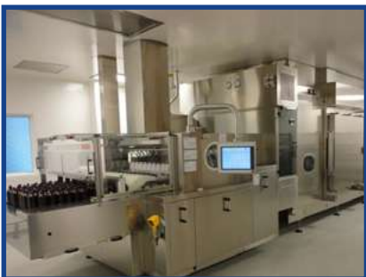
Line 10 Washer & Tunnel Washes, sterilizes and cools vials automatically.
